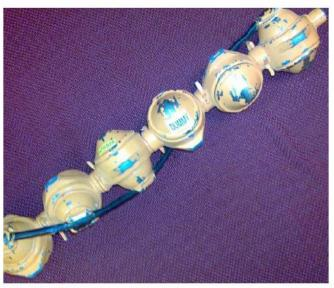
The new articulated chain gun system utilizes an encapsulated steel charge mounted on an expendable Zamac alloy connector. It is an ultra high performance expendable gun system for through-tubing applications. The system provides a more powerful explosive load than equivalent diameter retrievable hollow carriers (scalloped carrier). The Wireline string and firing head are recovered after perforation.
